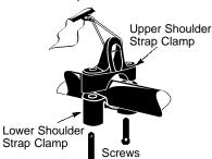
4 Insert two screws into the screw holes. Secure shoulder strap clamp by tighten-ing screws with a hex wrench. 5.
